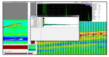
Advanced Data Analysis – Interactive histograms instantly reveal precise thickness measurements across scans.
