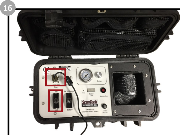
Open the lid and connect the power cable to the WS3 and connect the other end to a wall socket or to the battery pack. Flip the switch to turn the pump on.
