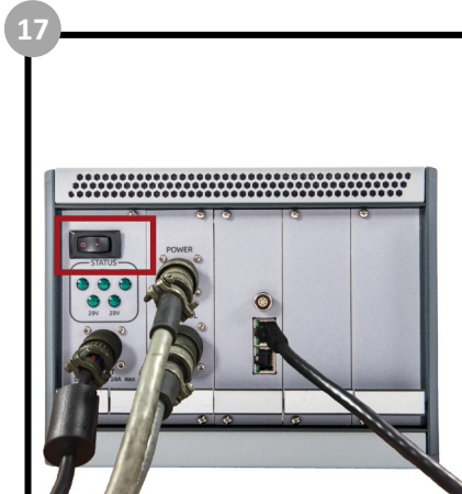
Turn on the controller box. The green lights beneath the power switch should all light up.
