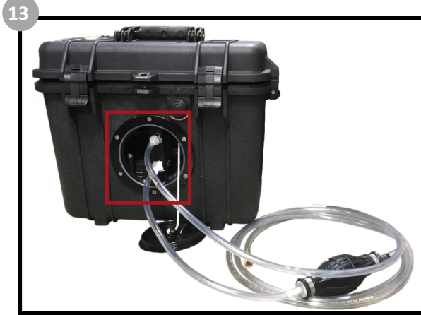
Remove the front panel of the WS3 and connect the hoses as shown.
