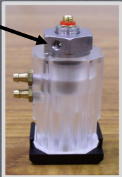
Set screw hold transducer into place
