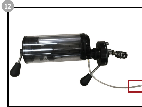
12 Connect the water hose (#8 - refer to the main cable assembly diagram) to the scanner.
