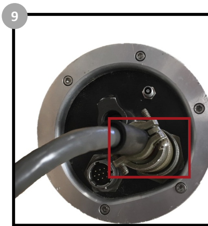
9 Connect the control cable (#7 - refer to the main cable assembly diagram) to the connection port on the scanner.
