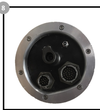
8 Locate the connection ports on the scanner for the main cable assembly.
