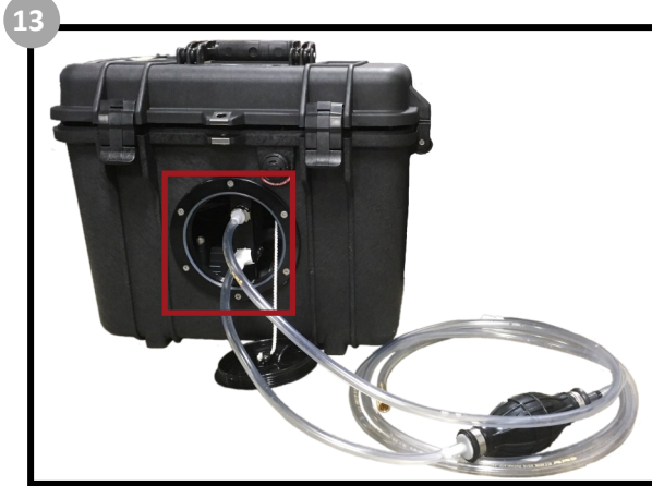
13 Remove the front panel of the WS3 and connect the hoses as shown.
