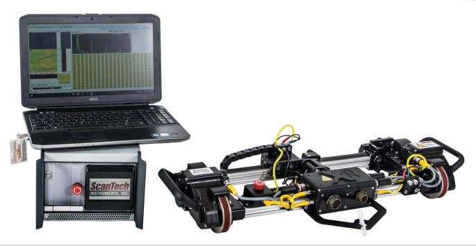
The XR Spider is an innovative ultrasonic scanner that addresses the need for an automated raster type unit. It offers higher performance and durability over an extended range of applications. The scanner traverses large vessels with obstacles that are problematic for most tank crawlers. It is capable of performing corrosion scanning on pipes as small as 2" while requiring no probe adjustments over the range.
