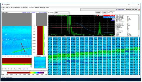
Optional: To change your view of the grid data, click and drag the red box on the C-scan data to the desired position.
