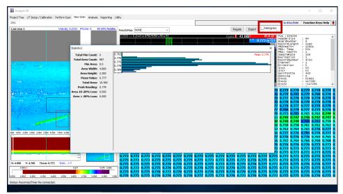
Optional: You can view a histogram of all of the data by click a checkbox in the upper right-hand corner. You can view a histogram of a selected region by clicking and dragging a box on your sample C-scan data.
