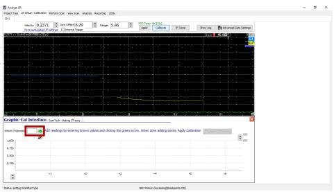
To calibrate, slide the UT instrument over the calibration block and enter the thickness of the block in the box labeled "Known Thickness:" and click the green arrow. Repeat this at a different thickness on the calibration block. If you need to remove data points, click the eraser button beneath the green arrow.
