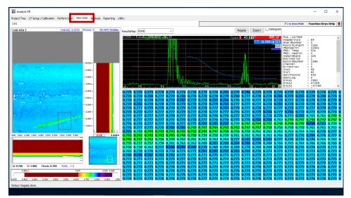
When the scan is complete, move to the "View Scan" Tab. At this point, you have the option to re-gate your data, create a histogram, export your data, or change the color mapping.
