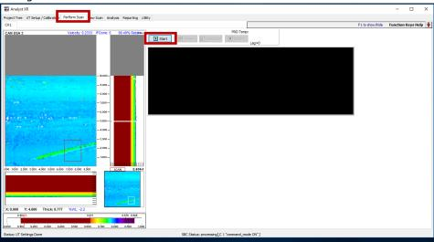
Next move to the "Perform Scan" tab. Once you have positioned your scanner, click "Start". Should you need to pause or stop the scan click "Pause" or "Abort". There is also an option to reposition the scan should there be an obstruction on the vessel. To do this, click "Reposition".
