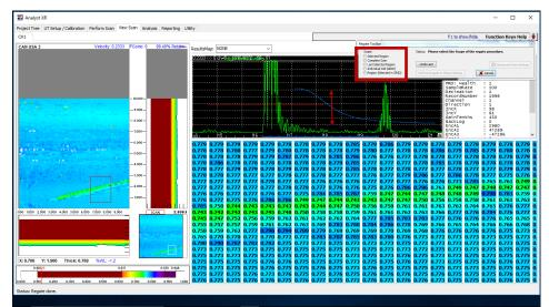
Optional: From this box select how many points you would like to regate: a single point, a selected region, or the entire scan. Select the points you are re-gating, and click and drag the gates on the A-scan to a new position.
