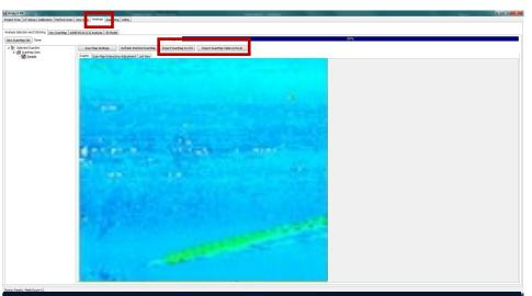
Next, move to the "Analysis tab". From this tab you have the option to stitch together multiple scans, perform ASME B31G analysis, generate a 3D model, and export data.
