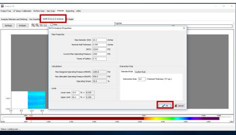
Optional: To perform ASME B31G analysis, click the tab and enter the properties of the pipe/vessel. Click "ok" to run the analysis.
