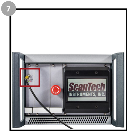
7 Connect the main cable wire (#4 - refer to the main cable assembly diagram) to the front of the controller box.
