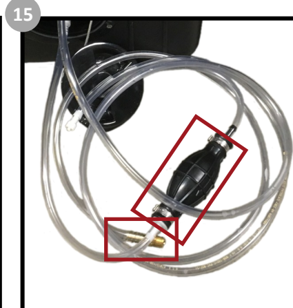
15 Connect the bottom hose to your water source. Turn on your water source and squeeze the pump to start the flow.
