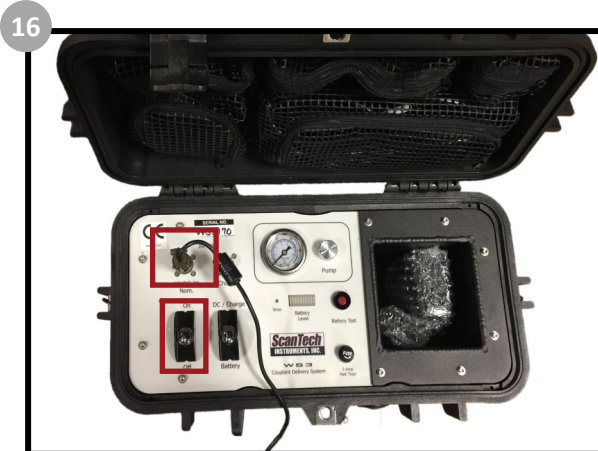
16 Open the lid and connect the power cable to the WS3 and connect the other end to a wall socket or to the battery pack. Flip the switch to turn the pump on.
