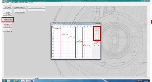
Optional: To compare multiple B-scan, click "Overlay B-scan View" and turn on and off different layers of the scan by clicking the different scans on the right side of the pop-up screen.
