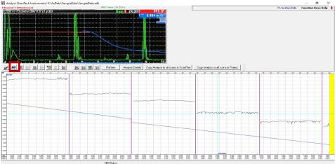
Optional: To add a clipping range, click the icon with the scissors. Then select the start and end of the range as well as the upper and lower limits; enter the high and low values and select "ok". This will remove any data outside of this range.
