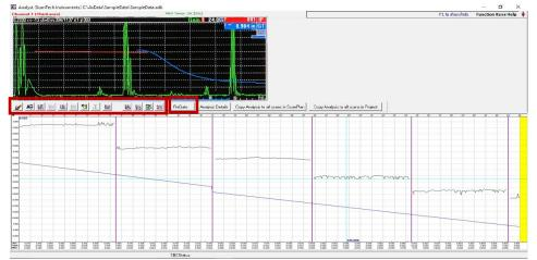
When the scan is complete, the tab should automatically switch to "Analysis". At this point, you can re-gate the data or perform statistical analysis.
