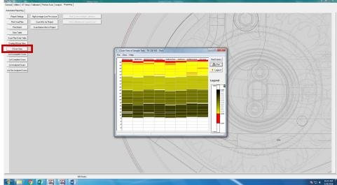
Optional: To generate a C-scan of the data, click "CScan View". This will automatically stitch together multiple B-Scans in a project to create a C-scan.
